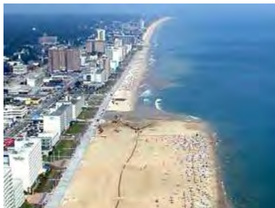
This photo, taken while the Virginia Beach Erosion Control and Hurricane Protection Project was underway, shows the significant difference between the unimproved area and the area of the widened beach berm already completed.
